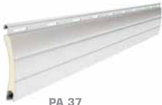
PA 37 Profile height: 37mm Thickness: 8,5mm
